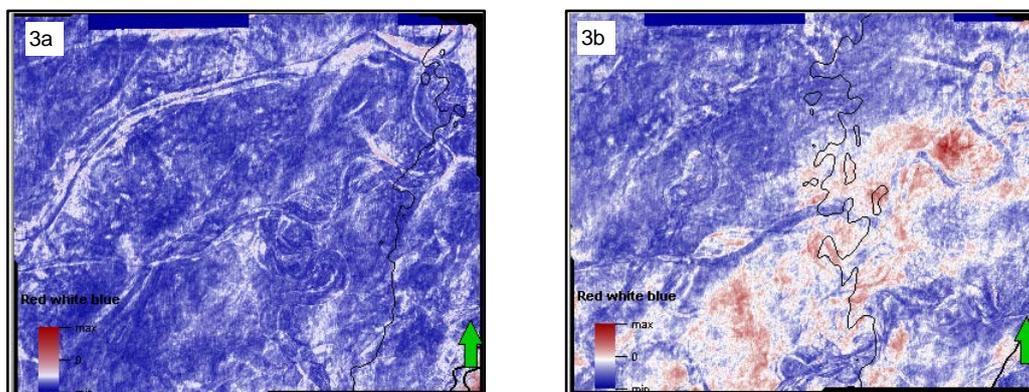
Figure 3: RMS Amplitude slices: a) Straight and meandering channels with feebly developed levees. b) Meandering channels and high amplitude over bank deposits.
