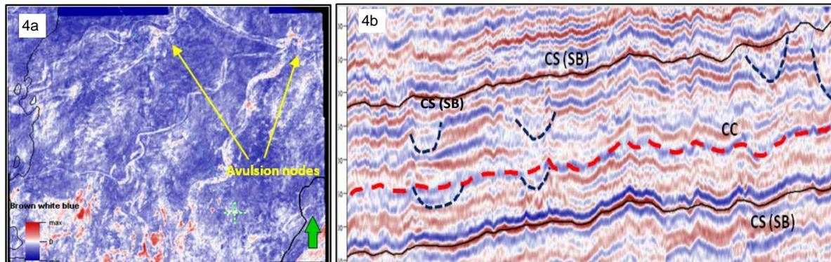
**Figure 4:** a) Avulsion nodes in northern parts of the area. b) Sequence 2: Dashed red line showing possible correlative unconformity, channels are marked in red.
