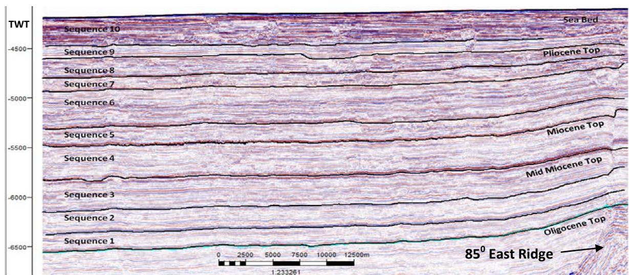
Figure 2: E-W Seismic section showing 10 sequences
