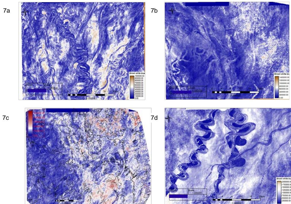
**Figure 7: RMS Slices a) SE flowing meandering channel cutting across southerly flowing relatively straight channels, sequence 7, b) Passive filling and general retrogradation of the system toward top of sequence 7 (20 ms above 7a), c) Pelagic interval above Pliocene top with a very high density of meandering shoe-string passively filled channels and d) Abandoned, entrenched channel levee complex cut by younger shoestring SW flowing channel, top of sequence 10.**
