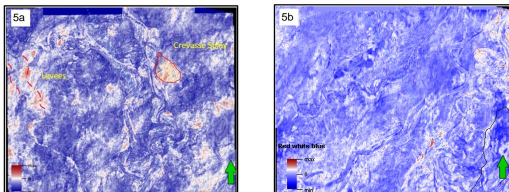
**Figure 5:** a) Map showing principally S flowing channels with levees and side lobes, the central channel shows SE flowing direction before taking Southward trajectory. b) SW flowing channels.
